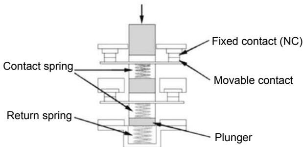
Both NC contacts incorporate a positive opening function. When metal deposition occurs, the contacts are separated from each other by pushing in the plunger.
