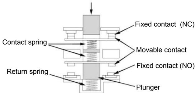
Only the NC contacts have a positive opening function. When metal deposition occurs, the contacts are separated from each other by pushing in the plunger.
